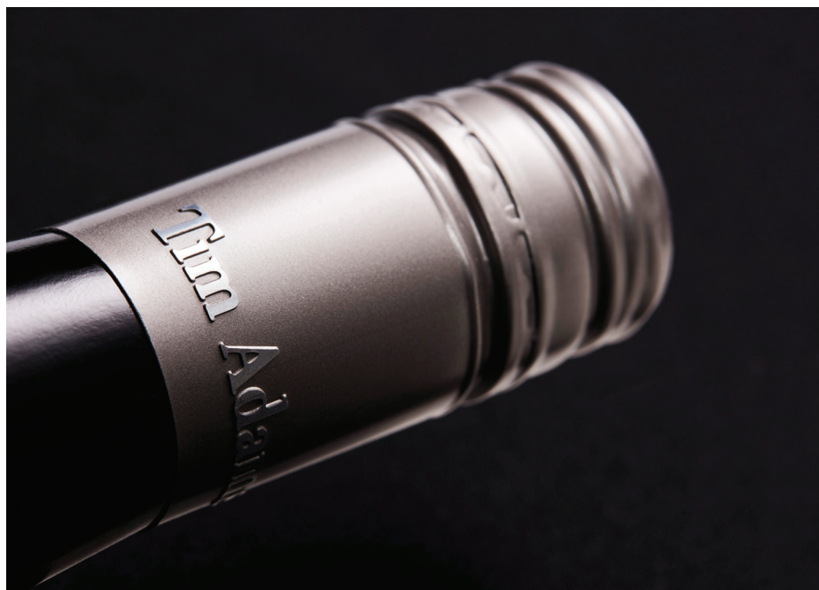
Shaved side embossing takes a standard blind emboss and shaves microns from the printed surface to reveal the aluminium beneath.
